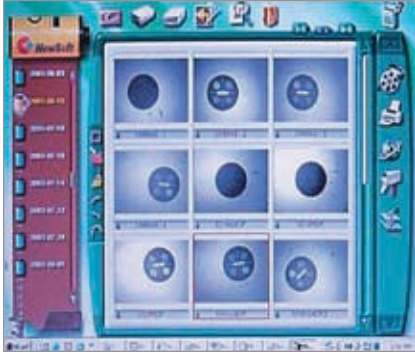
Fiber end images displayed on a PC
